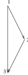
Fig. 2. This figure shown a network with 3 vertices. Vertex 1 is the source and vertex 3 is the destination. The following table shows the transmission and reception at various nodes for L = 3 messages.
